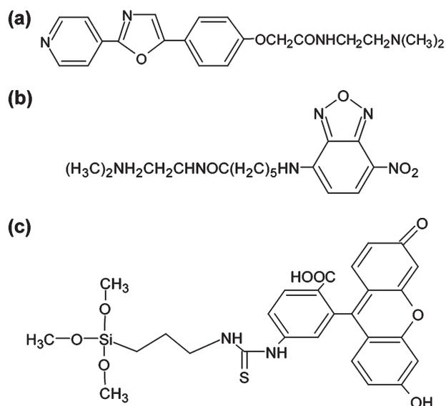
**Fig. 1** Chemical structures of the principal dyes used in this work. (a) DND-160 ( $C_{20}H_{22}N_4O_3$ ), also called PDMPO (for 2-(4-pyridyl)-5-((4-(2-dimethylaminoethylamino-carbamoyl)methoxy)phenyl)oxazole); (b) HCK-123 ( $C_{16}H_{24}N_6O_4$ ); (c) fluorescein-5-isothiocyanate (FITC)-silane.
