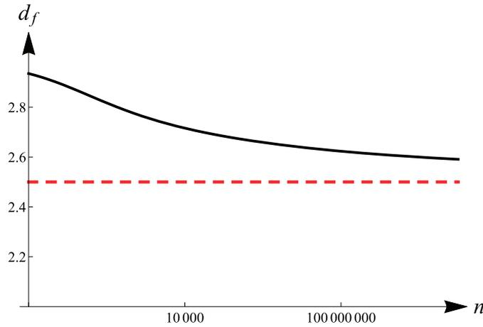
**Figure 4.** Solution (black curve) in  $d_f$  of the equation (33) versus the variable  $n$ . The red dashed line is the special value  $d_f = 5/2$ . The asymptotic solution for  $n \rightarrow \infty$  is  $d_f \simeq 5/(2 - \log 6/\log n) \rightarrow 5/2$ . This figure shows that, for any given value of  $d_f$ , the inequation (32) has solution in  $n$  only if  $d_f > 5/2$ .
