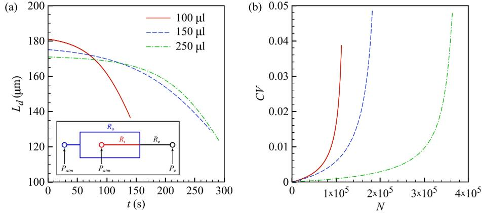
FIG. 4. (a) Model prediction of the time evolution of the droplet's length for the same suction volumes  $dV$  reported in Fig. 3. Inset: Schematic of the microsystem introducing the three hydrodynamic resistances considered in the model as well as the pressure condition at the inlets and outlet. (b) Model prediction of the coefficient of variation CV of the drop size as a function of the number of droplets collected in the exit micropipette's tip for the same conditions as in Fig. 4(a).
