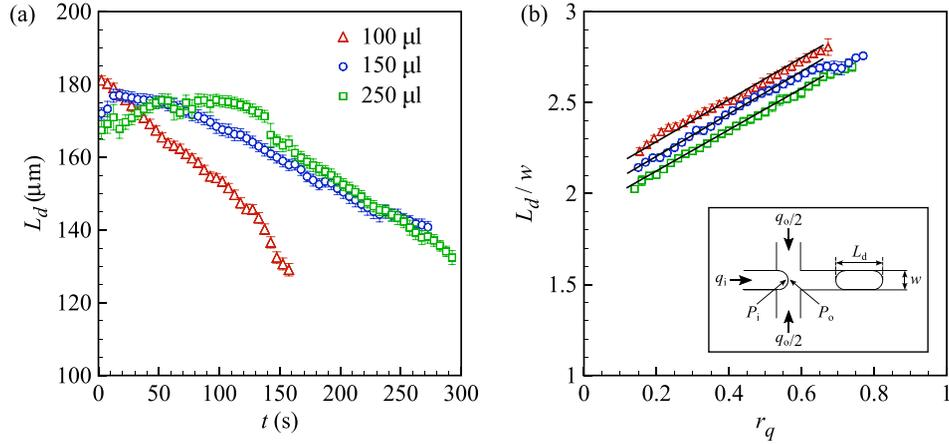
FIG. 3. (a) Time evolution of the droplet's length for various suction volumes  $dV$ . (b) Corresponding correlation between the droplet's length normalized by the channel's width as a function of the ratio between the flow rate of the inner phase and the outer one. Inset: Schematic of the cross-junction where droplets are formed along with flow and geometrical parameters.
