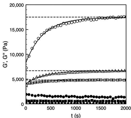
**Fig. 1** Time evolution of the elastic modulus  $G'$  (empty symbols) and the viscous modulus  $G''$  (filled symbols) of a natural rubber and carbon black mixture ( $\phi_{NR} = 0.22$  and  $\phi_{CB} = 0.028$ ) for three SDS concentrations: 16.5 mM (○, ●), 17.4 mM (△, ▲) and 17.8 mM (□, ■). The continuous lines reveal an exponential relaxation of  $G'$  towards its equilibrium value  $G'_m$  indicated by horizontal dashed lines.
