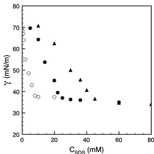
**Fig. 3** Surface tension of carbon black dispersions as a function of the SDS concentration for various volume fractions of particles: (○)  $\phi_{CB} = 0$ , (●)  $\phi_{CB} = 0.028$  and (▲)  $\phi_{CB} = 0.056$ .
