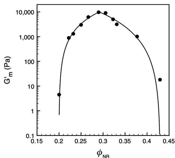
**Fig. 4** Plateau values of the elastic modulus  $G'_m$  of natural rubber and carbon black mixtures as a function of the NR volume fraction for fixed CB and SDS contents ( $\phi_{CB} = 0.028$  and  $C_{SDS} = 18.1$  mM). The curves represent critical-like functions.
