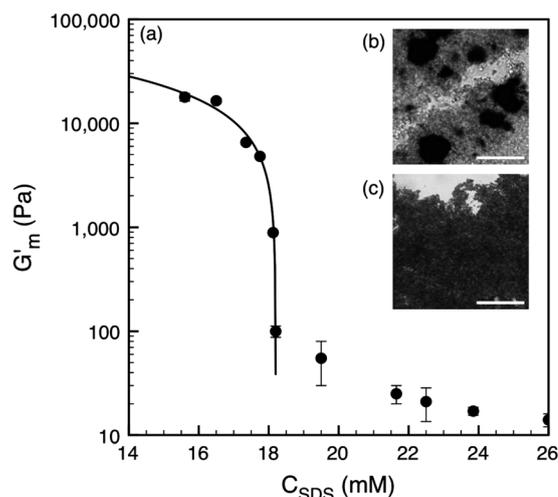
**Fig. 2** (a) Plateau values  $G'_m$  reached by the elastic modulus of a natural rubber and carbon black mixture ( $\phi_{NR} = 0.22$  and  $\phi_{CB} = 0.028$ ) as a function of the SDS concentration  $C_{SDS}$  in the binary colloidal dispersions. The curve is a critical-like function reflecting a gel–elastic solid transition. Pictures taken under a microscope of the mixture with SDS concentrations equal to (b) 15.5 mM and (c) 17.5 mM. The scale bars are 50  $\mu\text{m}$ .
