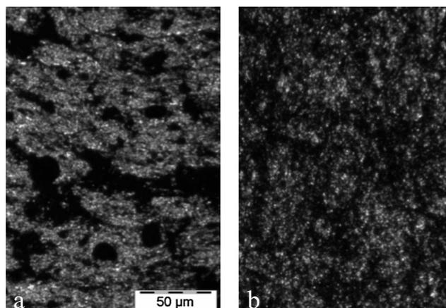
**Fig. 7** Pictures observed under a microscope with reflected light of the surface of dried coagulum slices: (a) without SDS and (b) with SDS. The final volume ratio between NR and CB is 4 and  $C_{SDS} = 16 \text{ mM}$ .
