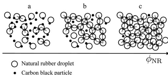
**Fig. 5** Sketches of the heteroaggregation process when the volume fraction of NR is increased while keeping the amount of CB constant. The gray lines show the networks formed by NR droplets bridged together with CB particles.
