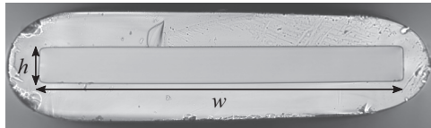
FIG. 1. Front view of a rectangular glass capillary having a height h of 96\ \mu\text{m} and a width w of 1050\ \mu\text{m} .
